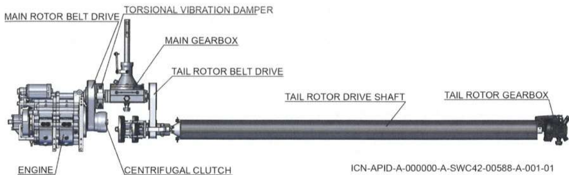
Figure 14 Main and tail rotor drive
